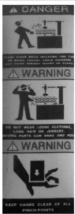
When rapid inflation, ensure the wheel clamped.
